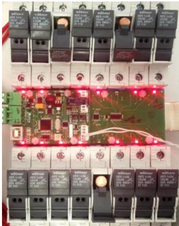
Figure 11. Sensor module indicating 13 of 16 circuits as active.
