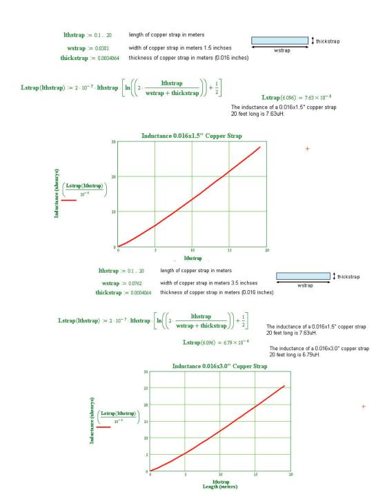
Simply increasing grounding strap width does not produce equivalent reductions in Inductance, and thus multiple point grounding straps are preferred.
