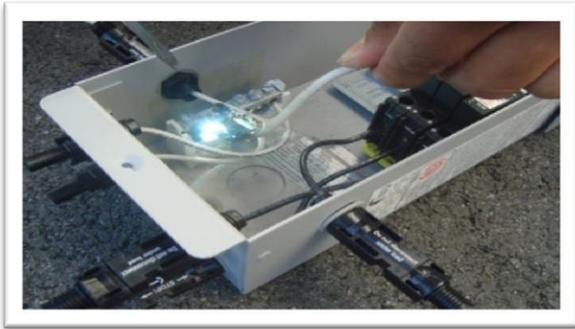
Figure 18 – Actual Arc Fault
