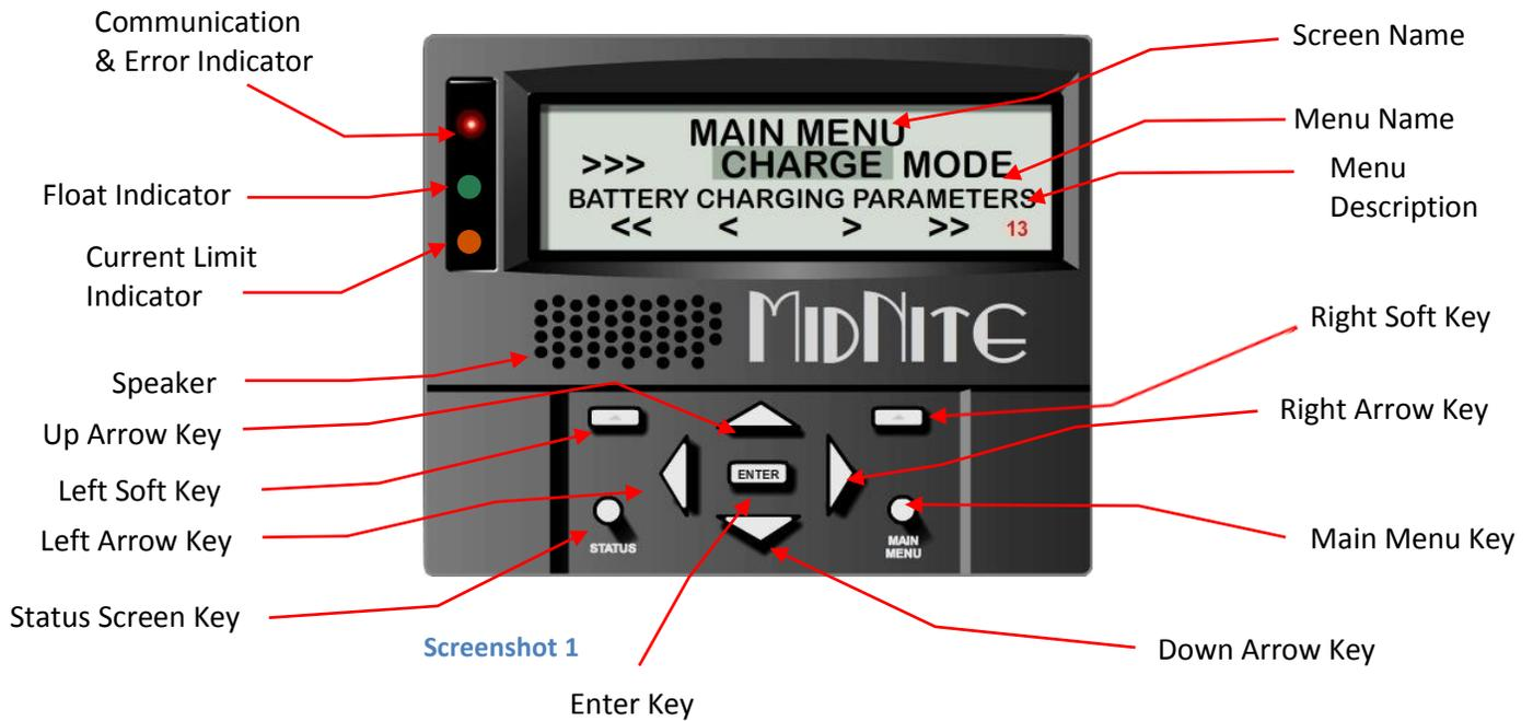
Most settings can be accessed and modified. Navigate using the LEFT and RIGHT ARROW keys. Pressing ENTER takes you into that menu. The MAIN MENU key also backs you out of any submenu. Use the soft-keys for options & views. Be sure to press ENTER to save changes before backing out of any menu/submenu.
