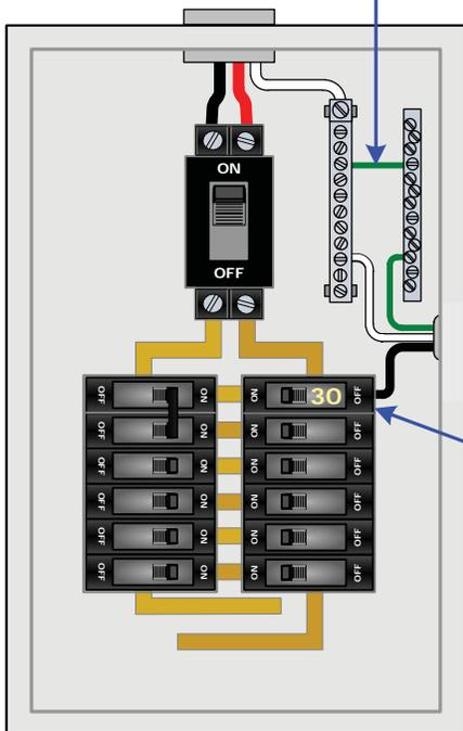
Maximum 30-amp breaker (single pole) required to invert AC input
