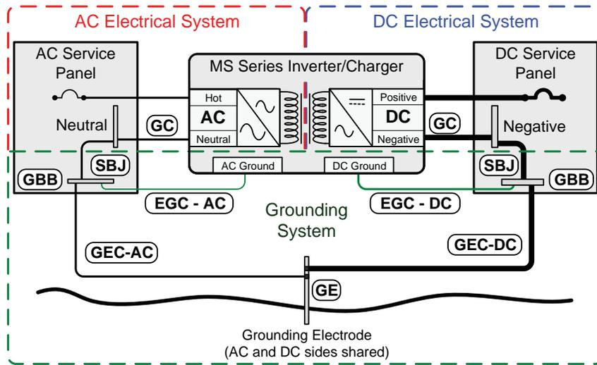
**Figure 2-18, Multiple Connections to DC Ground Rod (Method 2)**
