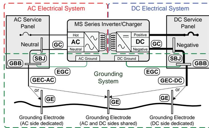
Figure 2-16, Grounding System for MS Series
