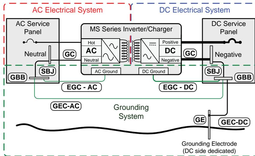
**Figure 2-19, Single Connection to DC Ground Rod (Method 3)**
