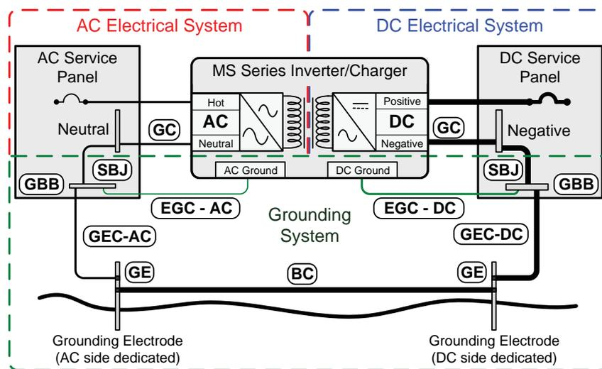
**Figure 2-17, Multiple Connections to DC Ground Rod (Method 1)**
