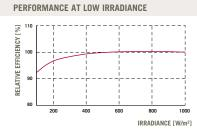
Typical module performance under low irradiance conditions in comparison to STC conditions (25  $^{\circ}\text{C},\ 1000\,\text{W/m}^2).$
