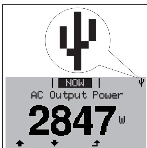
When the inverter recognizes a USB stick, the USB symbol will appear at the top right of the display.
