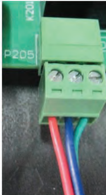
Figure 3-35 The dry contact communication cable connection
