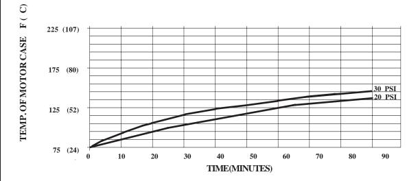
THIS GRAPH IS FOR USE AS A DESIGN GUIDE. IT IS BASED ON RUNNING CONTINUOUSLY WITH AN AMBIENT TEMPERATURE OF  $75^{\circ}$ F IN STILL AIR. THE THERMAL BREAKER WILL OPEN WHEN THE CASE TEMPERATURE REACHES  $210^{\circ}$ F.
