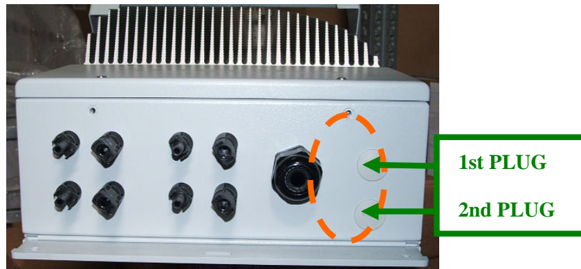
Fig.23 - Holes for cables necessary for RS-485 port connection or wiring for RJ12 connectors connection.
