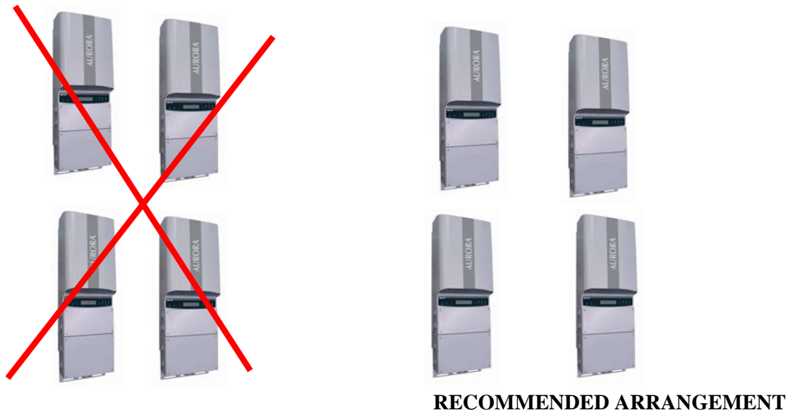
Fig.6 - Recommended installation of AURORA inverters
