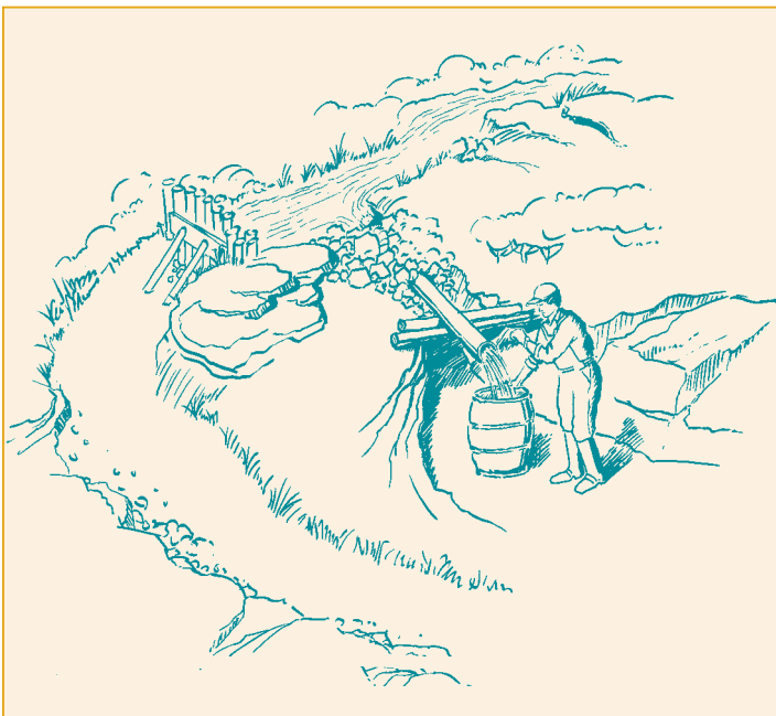
Figure 35. Measuring water flow rate using container method
