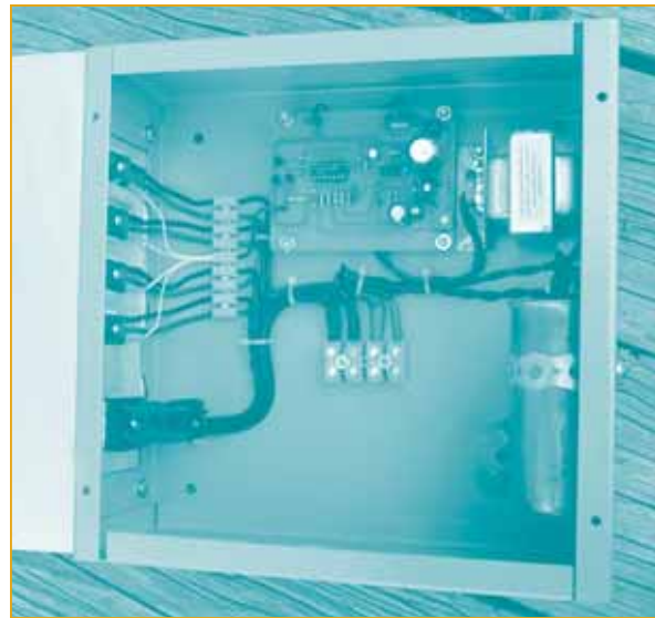
Figure 22. Induction generator controller, 3-kW rated (photo courtesy of Homestead Hydro Systems)
