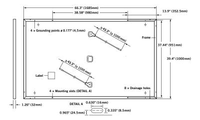
Fig. 1: External dimensions (in inch (mm)) and components for Q.PEAK DUO-G5.X, Q.PEAK DUO BLK-G5.X,
