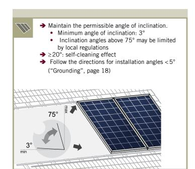
Fig. 2: Installation options for crystalline Q CELLS modules. All dimensions are given in inch (mm in brackets). Also observe the maximum test loads and clamping range as specified on the following page. The illustrated installation options apply for both horizontal and vertical module orientation.
