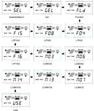
Note: If the controller supports 48V system voltage, the battery type will display LiFePO4 F15/F16, and Li(NiCoMn)O2 N13/N14.
