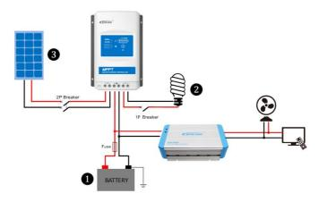
Figure 2-2 Schematic of wiring diagram
