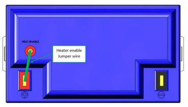
Figure 4: Heat Enable Jumper Wire Setup
