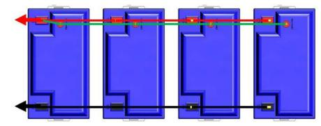
Figure 14: Heat Enable daisy chained in 12V parallel
