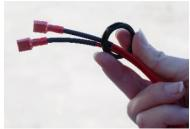
Figure 9: Heat Battery Kit harness through plastic nut
