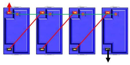
Figure 16: Heat Enable daisy chained in 48V series
