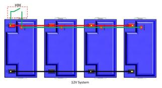
Figure 8: 12V daisy chained enable wires set up in parallel
