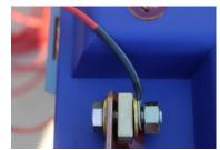
Figure 12: Bolt, washer, battery cable, positive terminal, washer, 5/16" heat enable wire, nylok
