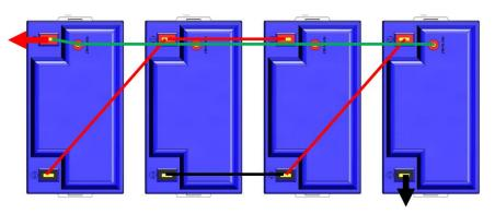
Figure 15: Heat Enable daisy chained in 24V series/parallel
