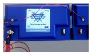
Figure 7: Top view of daisy chained heat enable post
